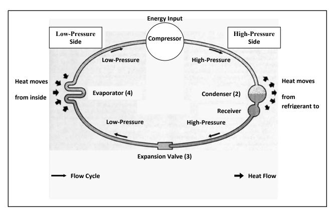
Figure 1-1 Complete Four-part Cycle of Air-conditioning
