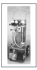
Figure 1-36 Refrigerant Servicing and Recycling Station
